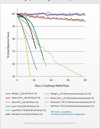
XBridge Columns resist base particle dissolution and ligand hydrolysis when used with high-pH mobile phases. No other column family has the extended lifetime of an XBridge HPLC Column at elevated pH.
