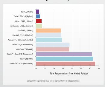
XBridge packings incorporate well-characterized, state-of-the-art bonding and endcapping procedures to provide columns that are more stable using acidic-pH mobile phases compared to conventionally prepared columns.
