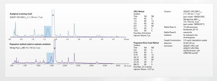
Scaling and optimization of preparative separations using XBridge Preparative OBD Columns. This example of a degradant isolation from ranitidine (API) (degradant highlighted in blue) shows that by maintaining column length to particle size ratio (L/dp), you can geometrically scale the separation to achieve a high sample load without compromising resolution.
