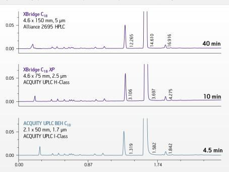
Make your HPLC system more productive with XP 2.5 µm Columns.. Unlike core-shell columns, methods developed on eXtended Performance 2.5 µm Columns can be scaled and transferred to larger 3.5 and 5 µm HPLC columns, or to smaller sub-2-µm UPLC Columns, providing flexibility and method consistency between laboratories.
