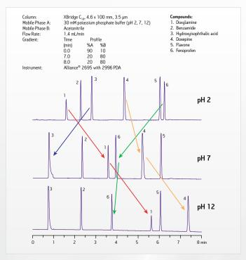
XBridge Columns are unique in their ability to withstand these aggressive conditions (even at pH 12) allowing complete flexibility for the method development chemist, while maintaining the highest efficiency values associated with silica columns.
