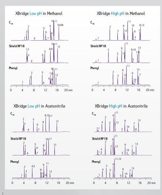
By systematically screening a standard set of conditions, the separation scientist can quickly determine the best starting point for further method optimization.
