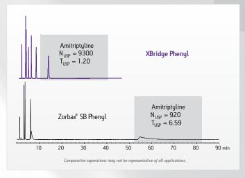
XBridge Phenyl Columns combine trifunctional bonding of the phenyl-hexyl ligand with proprietary end capping to produce industry-leading stability and exceptional peak shape.
