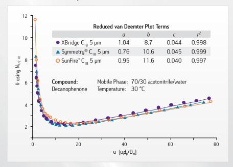
The reduced plate height, h, is a function of the reduced linear velocity, v, (both normalized for particle size) and a, b, and c summarize the contributions of eddy diffusion, longitudinal diffusion, and the sum of stationary- and mobile-phase mass transfer terms, respectively.
