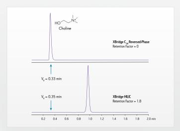
XBridge HILIC Columns provide retention for polar compounds that are too weakly retained using a traditional reversed-phase method.
