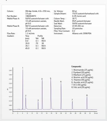
Very polar compounds, such as water soluble vitamins, are easily retained and separated using an XBridge Amide HPLC Column. The high-pH mobile phase ionizes the acidic compounds to provide more interaction between the amide ligand and analyte.
