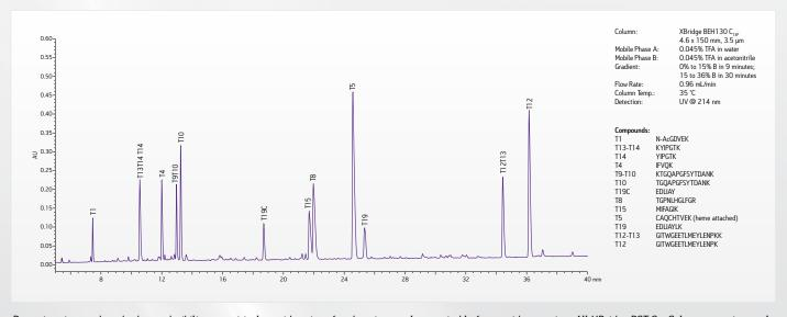
Retention time and method reproducibility are critical considerations for choosing a column suitable for peptide mapping. All XBridge PST  $C_{18}$  Columns are rigorously tested using a QC sample based on a tryptic digest of bovine cytochrome c. This insures that the column provides peptide separations spanning a broad range of hydrophobicity isoelectric points.
