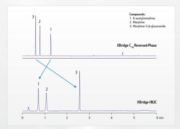
XBridge HILIC Columns provide orthogonal selectivity when compared to reversed-phase HPLC columns. As seen here, the polar metabolites of morphine are retained longer under HILIC conditions (vs. a reversed-phase separation).
