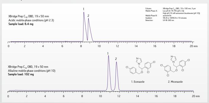
On column sample loading for basic compounds can often be increased by using high-pH mobile phases. As this example shows, conventional methods using acidic mobile phases and ion-pairing reagents provide inferior load, retention, and resolution compared to the same method using a high-pH mobile phase.
