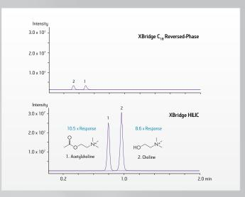
XBridge HILIC provides enhanced mass spectrometry response resulting in lower limits of detection.
