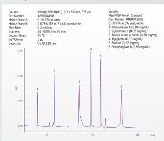
XBridge BEH300  $C_4$  Columns can be used with proteins that have a wide range of properties. This protein mix was chosen to represent a range of isoelectric points, molecular weights, and hydrophobicities.
