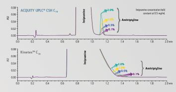
The improved mass loading of XSelect columns permits the separation, identification and quantification of closely eluting impurities or degradants.
