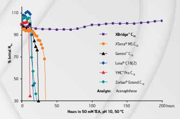
Accelerated High pH Stability Test of Competitive Columns
