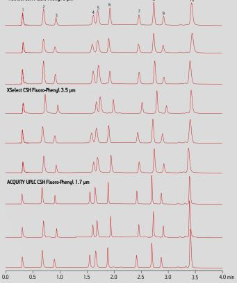
Reproducibility and scalability for gradient separations on 2.1 x 50 mm columns containing nine different batches of CSH Fluoro-Phenyl representing three (1.7, 3.5, and 5 µm) particle sizes. Compounds: [1] thiourea, [2] resorcinol, [3] metoprolol, [4] 3-nitrophenol, [5] 2-chlorobenzoic acid, [6] amitriptyline, [7] diethylphthalate, [8] fenoprofen, [9] dipropylphthalate, [10] pyrenesulfonic acid.
