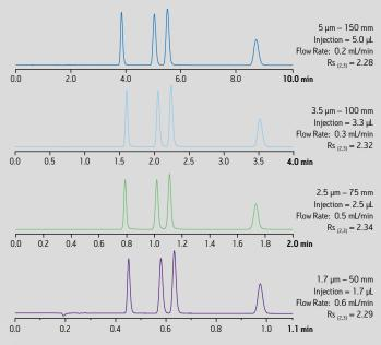
Columns of different lengths and particle sizes were used to successfully reduce run times and maintain resolution.
