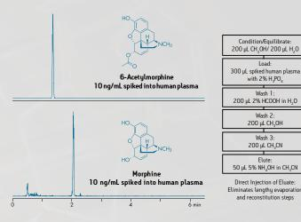
XBridge HILIC provides direct injection of SPE eluents, thus increasing sample throughput.
