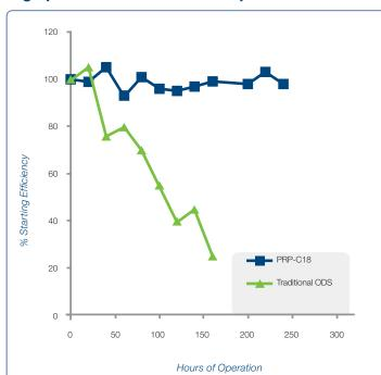
Forced degradation study comparing resilience of traditional ODS C18 and Hamilton PRP-C18 Reversed-Phase HPLC Columns. Efficiency monitored periodically while columns were purged at 1 mL/min with 50% acetonitrile containing 50 mM potassium phosphate, pH 12.
