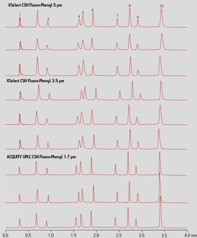
Reproducibility and scalability for gradient separations on 2.1 x 50 mm columns containing nine different batches of CSH Fluoro-Phenyl representing three (1.7, 3.5, and 5  $\mu$ m) particle sizes. Compounds: [1] thiourea, [2] resorcinol, [3] metoprolol, [4] 3-nitrophenol, [5] 2-chlorobenzoic acid, [6] amitriptyline, [7] diethylphthalate, [8] fenopropfen, [9] dipropylphthalate, [10] pyrenesulfonic acid.
