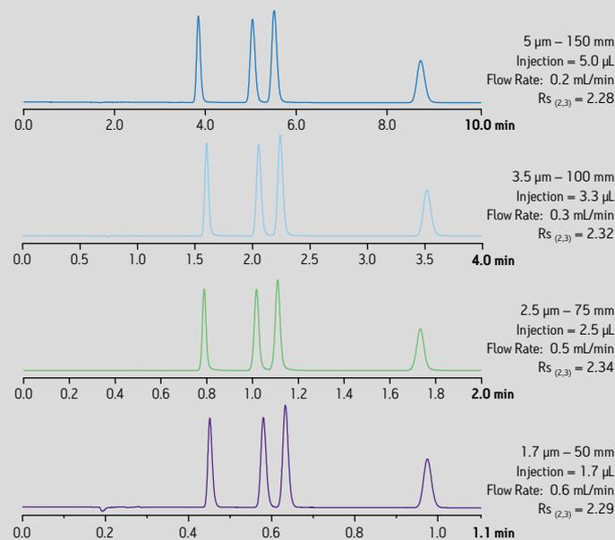
Columns of different lengths and particle sizes were used to successfully reduce run times and maintain resolution.
