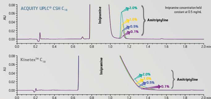
The improved mass loading of XSelect columns permits the separation, identification and quantification of closely eluting impurities or degradants.
