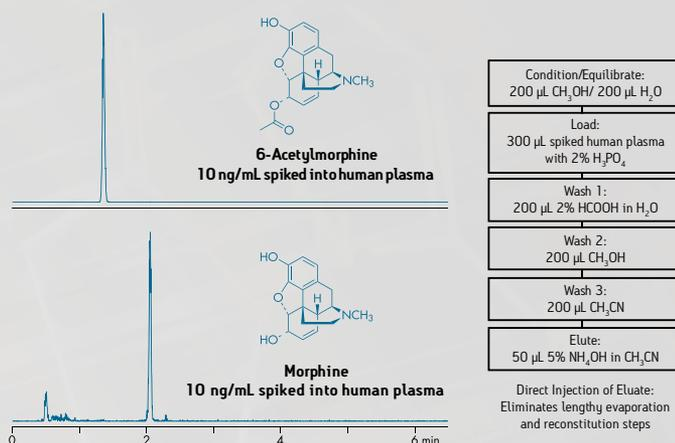
XBridge HILIC provides direct injection of SPE eluents, thus increasing sample throughput.
