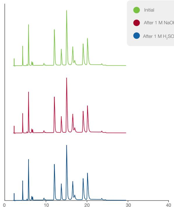
Separation of standard mix after 200 column volumes 1 M NaOH and 1 M H<sub>2</sub>SO<sub>4</sub>.
