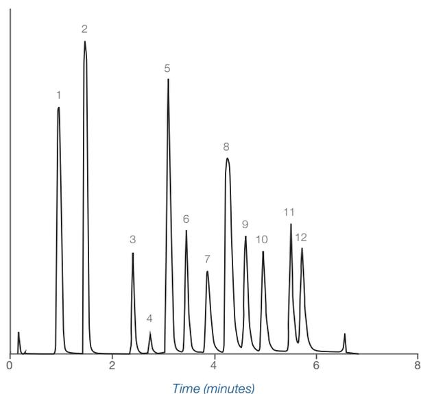
Separation of 12 standards in a short, 5 minute linear acetonitrile gradient.
